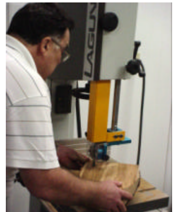
Ken Goldspink cutting a bowl blank on our new laguna band saw
