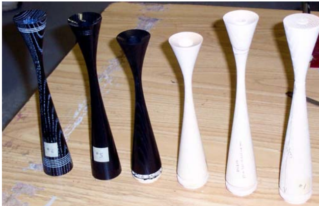
Martin Groneng candlesticks shown at the various stages with the finished product on the left
